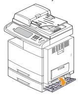
Pull the jammed paper out in the direction shown. To avoid tearing the paper, pull it out gently and slowly.
